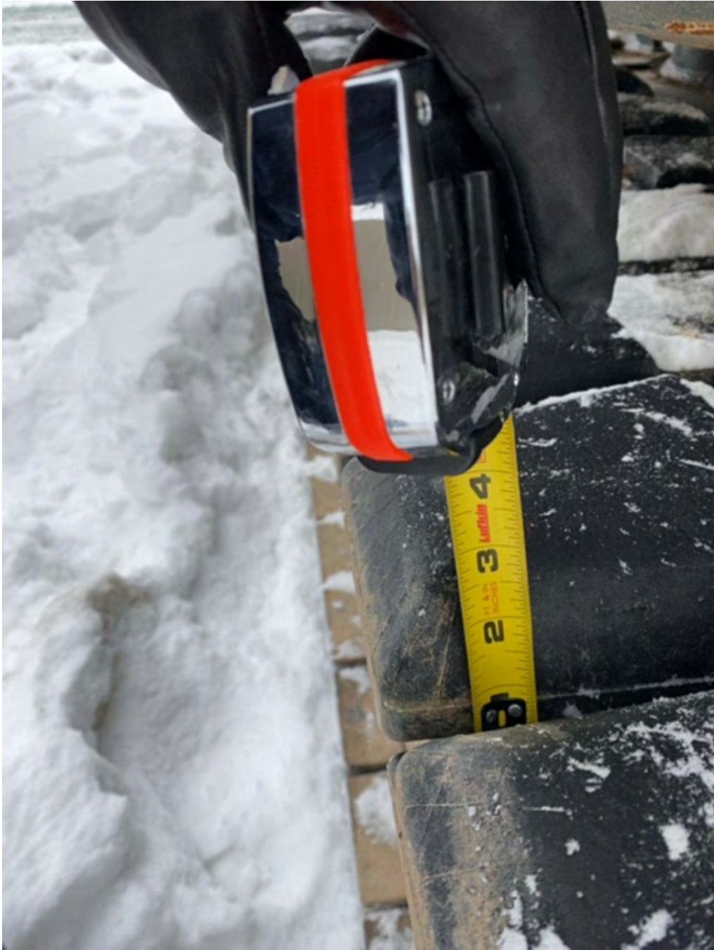
Left Track Tread Depth Measurement / 02-15-2021
