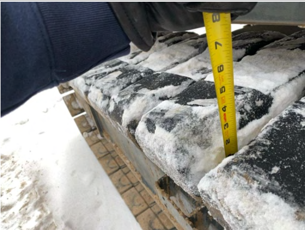
Right Track Tread Depth Measurement / 02-15-2021
